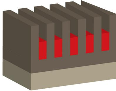
After a dye has been embedded into these pores, you can again close the oxide layer by the so-called sealing. This means that aluminium oxide reacts with water and crystallizes to hydrate alumina ( $\text{Al}_2\text{O}_3 \times \text{H}_2\text{O}$ ) which clogs the pores.
