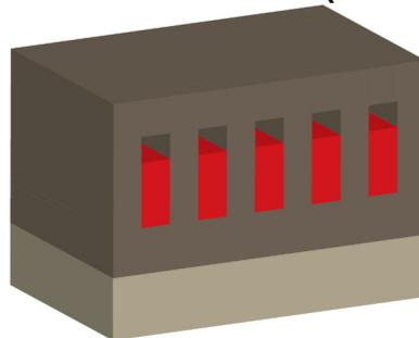
The dye is thereby permanently bound to the aluminium and cannot be scraped off or flake like varnishes for example. It is of course also possible to not embed any dye or to seal the oxide layer directly after anodizing; then, the work piece keeps its silvery grey colour yet is nevertheless protected against corrosion.
