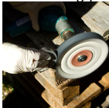
You see the increasing mirror-like gloss come to light. After the polishing, the surface has darkened areas which are easily removed by a cloth and some water.
