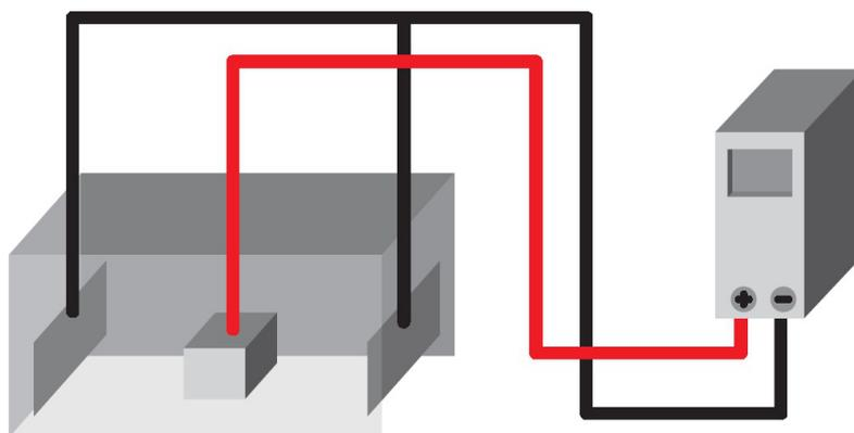
Attach the 2 stainless steel anodes (cathodes) supplied along the 2 long sides of the tub or in a suitable vessel. The arrangement with 2 cathodes around the workpiece has the advantage of a better current density distribution. The aluminium workpiece is connected as an anode i.e. it is connected to the positive pole!
